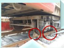
The vehicles/ load/ train be chained and padlocked using at least two chains, one at either end.
